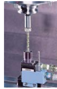
Touch Type In-Process TLM Measurement + Broken Tool Detection + Auto Centering
