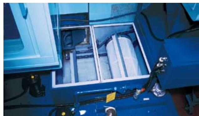
Drum Filter for the Lift-up Chip Conveyor
